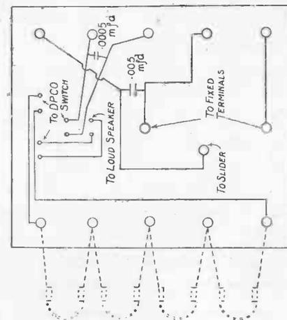
Fig. 97.—Wiring of End Panel with Four Pairs of Phones in Series.
