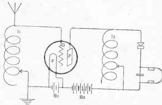
Fig. 8.—Valve as High-frequency Amplifier with Crystal Detector.
