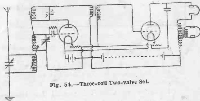
Fig. 54.—Three-coil Two-valve Set.
