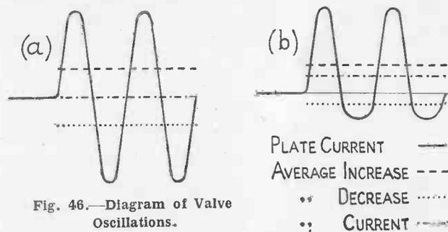
Fig. 46.—Diagram of Valve Oscillations.
