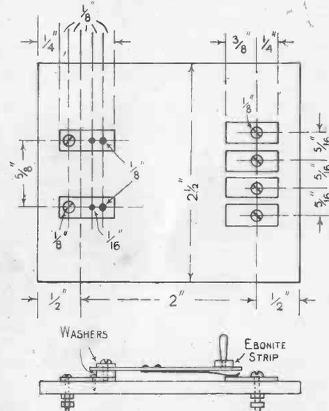
Fig. 63.—Details of Switch.
