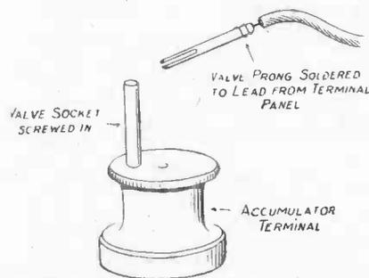
Fig. 81.—Detail of Accumulator Terminal with Valve-socket Connector.
