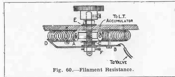
Fig. 60.—Filament Resistance.
