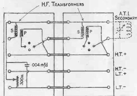
Fig. 107.—Potentiometer Connections of H.F. Transformer Panels.
