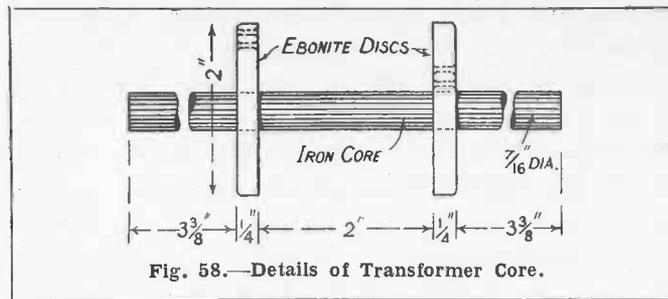
Fig. 58.—Details of Transformer Core.
