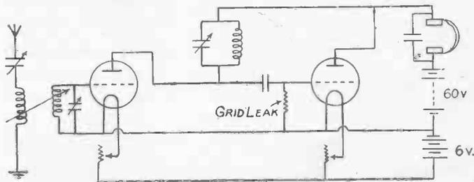
Fig. 83.—Tuned-anode Coupling of H.F. to Rectifying Valve.
