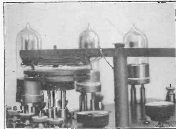
Fig. 64d.—Photograph showing Reaction Coil.
