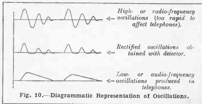
Fig. 10.—Diagrammatic Representation of Oscillations.
