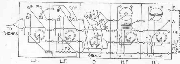
Fig. 113.—Wiring Diagram of Improved Set.
