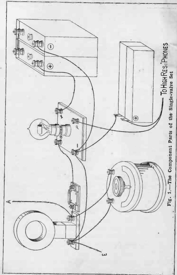
Fig. 1.—The Component Parts of the Single-valve Set
