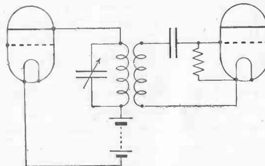
Fig. 48.—Connections of H.F. Transformer.
