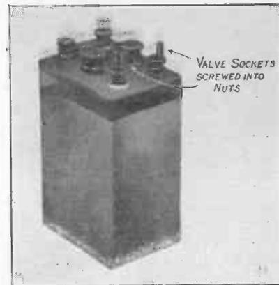
Fig. 80.—Photograph of Accumulator with Valve Sockets Fitted to Terminals.
