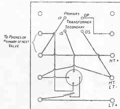
Fig. 91.—Wiring Diagram of Low-frequency Panel.
