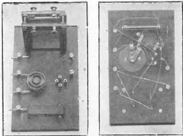
Fig. 111.—Upper and Under Views of Low-frequency Panel.
