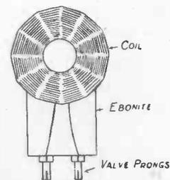
Fig. 76.—Detail of Coil Holder with Coil.
