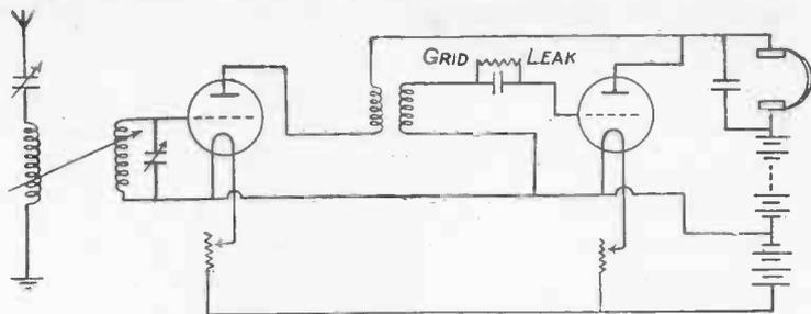
Fig. 82.—High-frequency Air-core Transformer Coupling.
