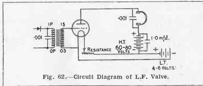
Fig. 62.—Circuit Diagram of L.F. Valve.
