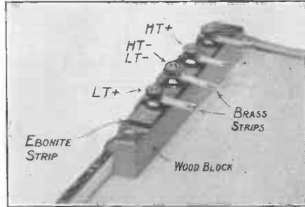
Fig. 71.—Photograph of Terminal Panel.
